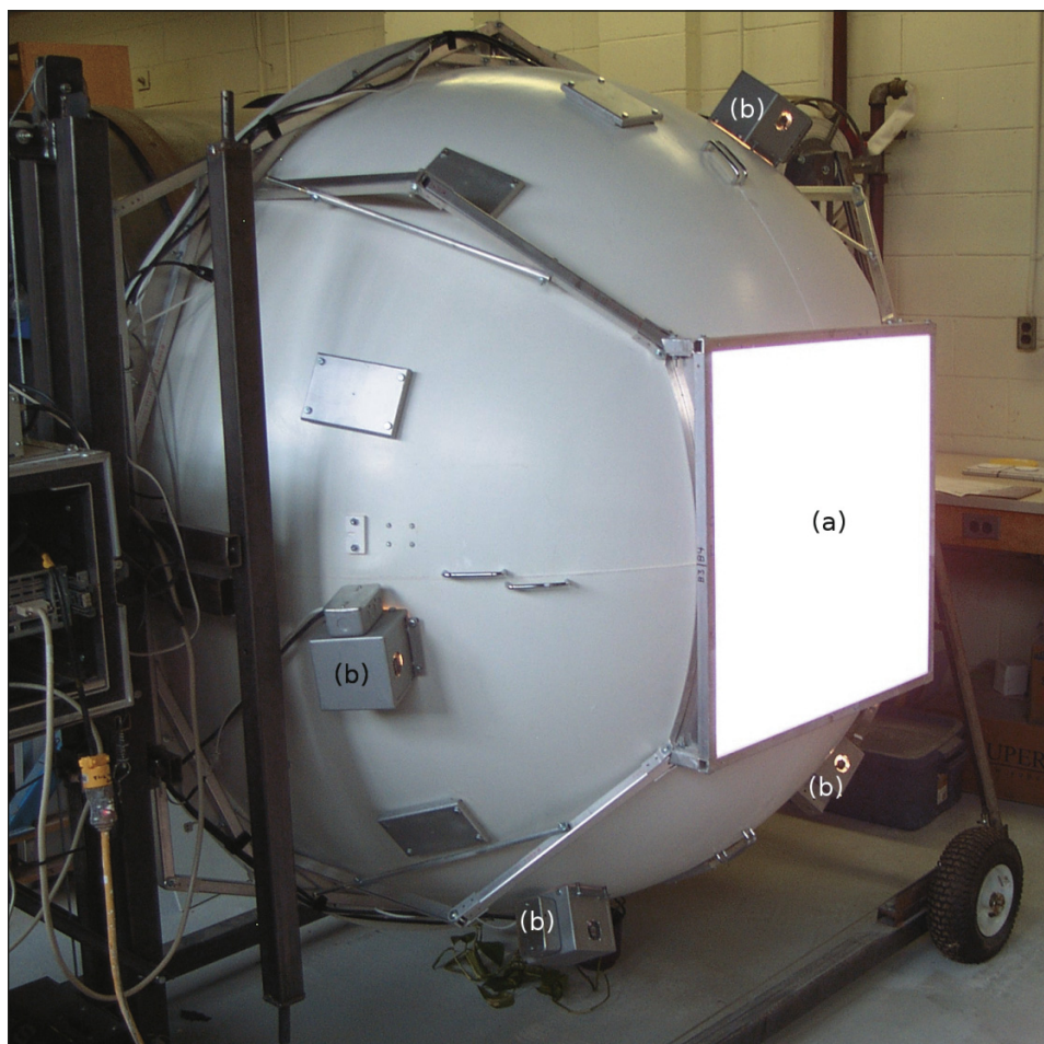
Figure 1. The 1.8 m integrating sphere for which the coating discussed in this paper was developed (Noble, 2006). The integrating sphere is configured as a uniform light source. The sample being illuminated is placed at the sample port (a), and the sphere interior is illuminated by a set of lamps (b). Integrating sphere theory dictates that a spherical interior geometry with a Lambertian coating will disperse incident light such that uniform intensity is experienced at all points of the surface.
